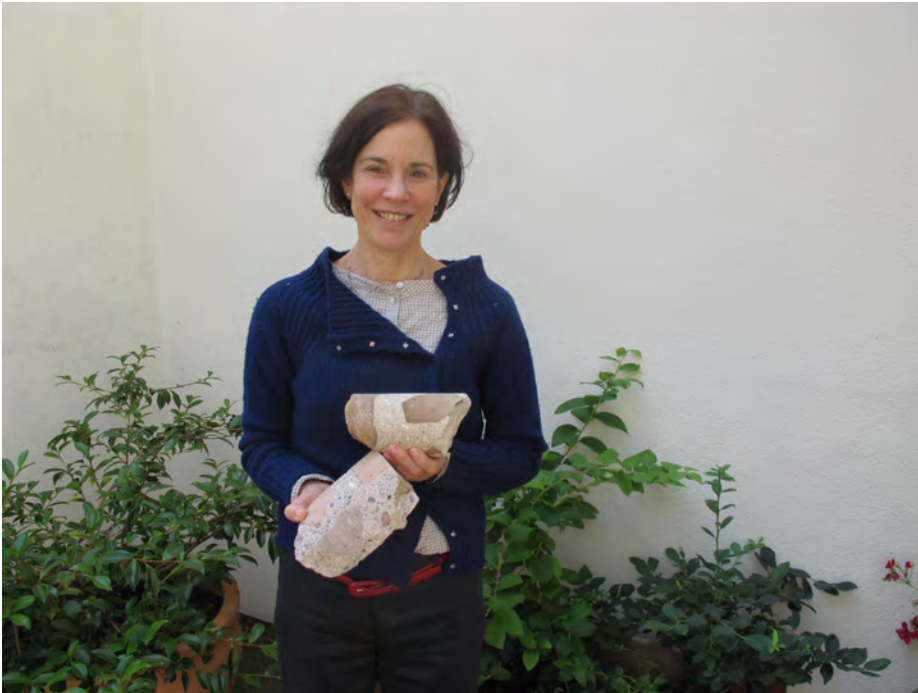
Figure 1. Marie Jackson holding ca. 1900-year-old concrete drill cores from Roman edifices constructed during the reign of Emperor Trajan (98-117 CE). The lower core at left is from the Markets of Trajan (~110 CE) in Rome, the one on the right is from Portus Traianus (~115 CE) in Ostia, about 15 km downstream along the Tiber River. Both contain tuff and brick coarse aggregates, but the mortars have different volcanic ash pozzolan and the hydration of lime and mortar mixing procedures were also very different. These are some of the very best architectural and harbor concretes that were made by imperial Roman builders.
