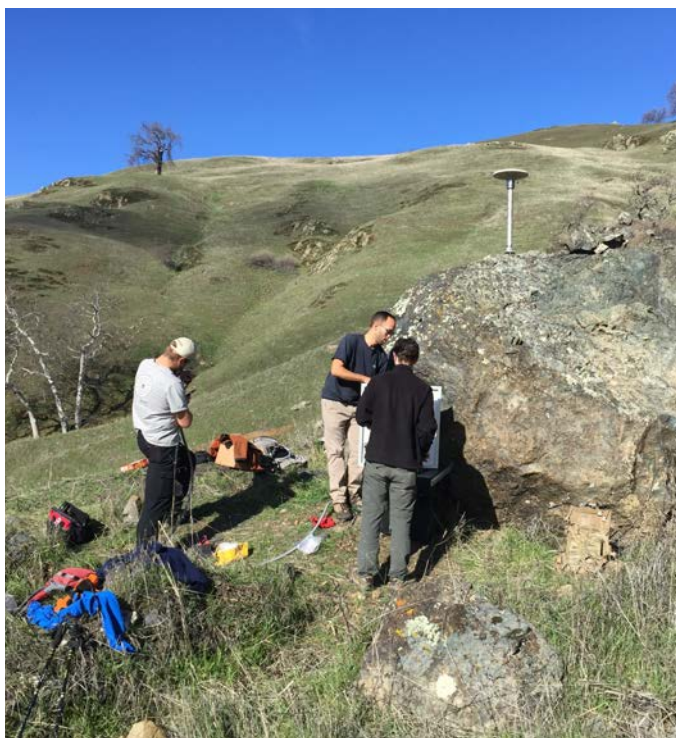
Grad student Alex Nereson and colleagues installing a continuous GPS station on a boulder in the Diablo Range earthflow, northeast of San Jose
