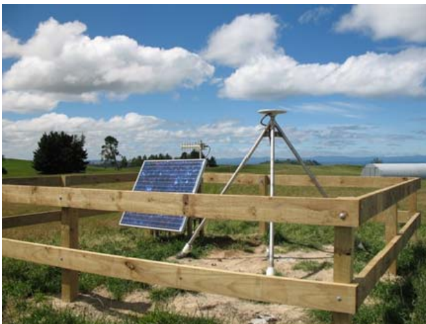
A continuous GPS site in the North Island, New Zealand that is part of the GeoNet cGPS network ( www.geonet.org.nz )
