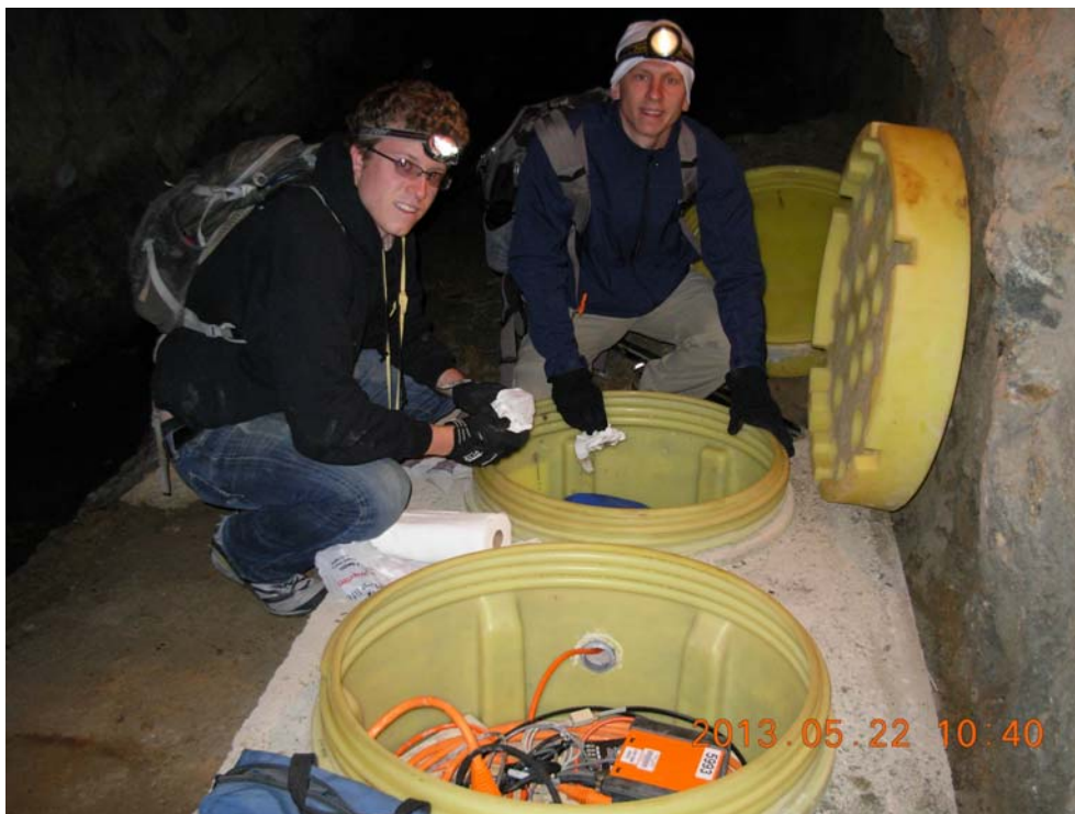
2013 USGS intern (and 2013 UCSC Earth Sciences graduate) Jonathan Ooms (on left), completing a routine check on one of the ANSS "backbone" seismic stations in Idaho Springs Colorado (ISCO). The large yellow vaults hold a broadband seismometer (background) and data acquisition system (foreground). The station is located 400ft inside a former mine tunnel.
