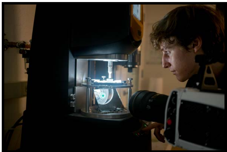
Undergraduate Jaden Zak in the Earthquake Physics lab modelling rupture and friction using scaled experiments.
