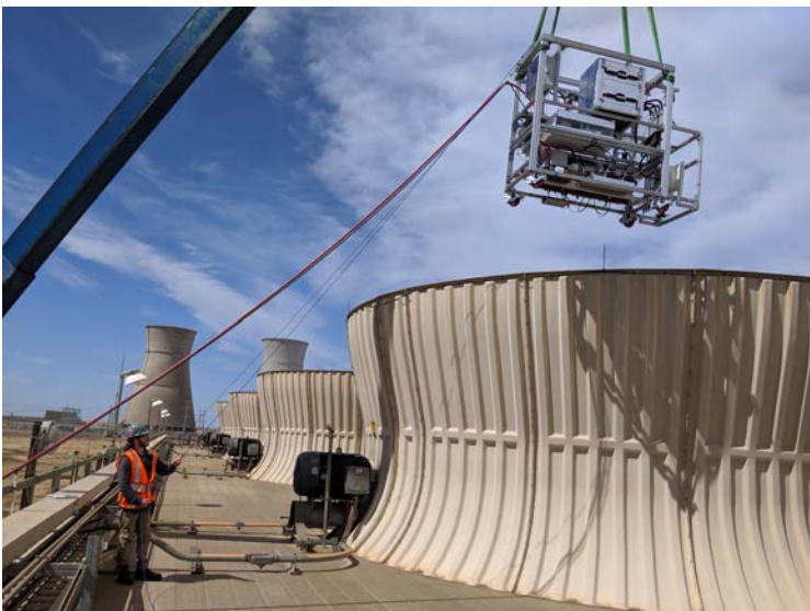
Equipment for monitoring droplet emissions in a power station cooling tower
